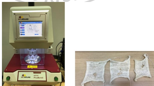
Figure 159 Pneumatic: Auto Mode (left) and fabric test sampling (right)
