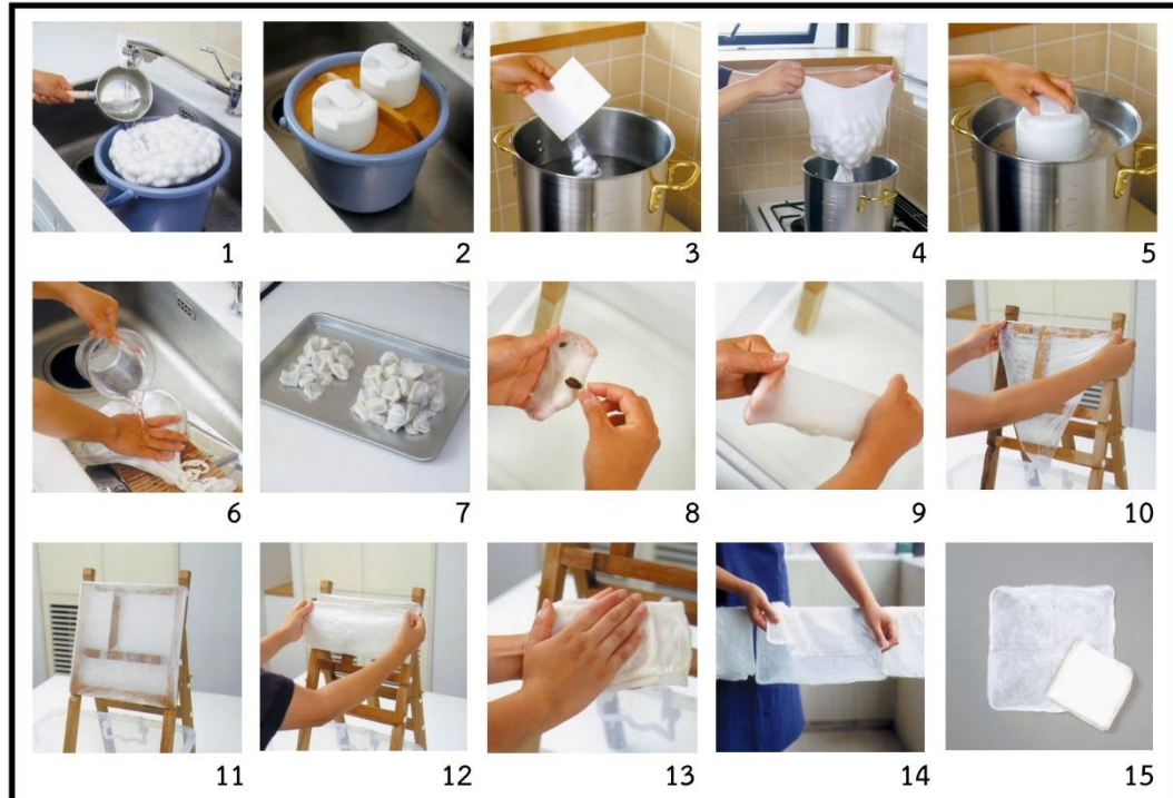
Figure 24 The mawata production. (Japan Floss Silk Association, 2016)
