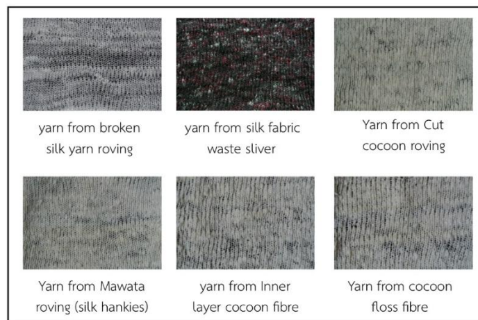
Figure 130 A fabric produce by domestic knitting machine: brother HK-386
