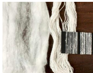
Figure 27 A sample of yarn from hand spinning: The noil top (left), the small neps or noils show up in the yarn as bumps of texture (center and right). (Sara Lamb, 2014: 80)
