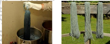
Figure 53 Immersion dyeing the skeins (left) and the result (right) (Barbara Parry, 2009: 74-77).
