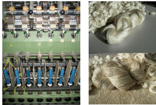
Figure 13 Ring spinning machine (left) (Roxanna Cody, 2012: 10) and a sample of yarn from machine spinning. (Mathias Camenzind and others, ed., 2014: 13)
