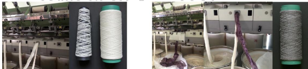
Figure 127 Open-end spinning machine, Yarn from cut cocoons sliver: cotton sliver was 50:50 (left) and open-end spinning machine, yarn from silk fabric waste sliver: cotton sliver was 50:50 (right)
