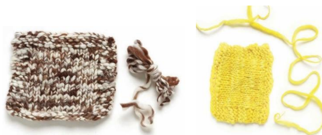
Figure 34A sample of Marled single yarn (left) and Thick-and-thin single yarn (right)(Amy King, 1973: 73-74).
