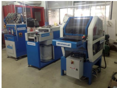
Figure 119 The MESDAN LAB laboratory carding machine serial number 137 (right) and the MESDAN LAB laboratory drawing machine serial number 21 (centre).
