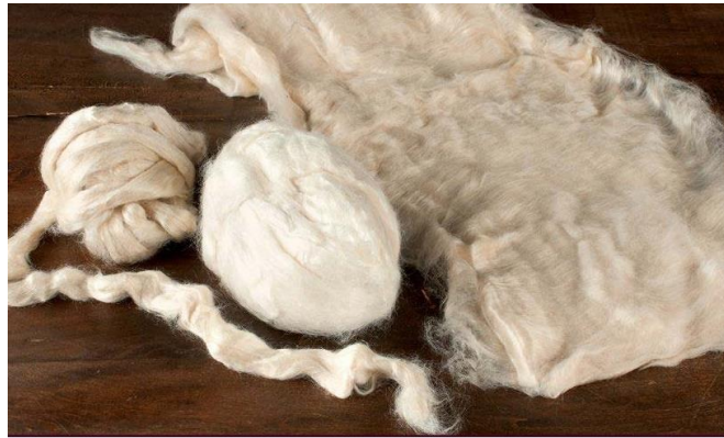
Figure 11 Silk fiber is available in many forms, including top (left), folded into a brick (center), or in laps (right). (Sara Lamb, 2014: 38)
