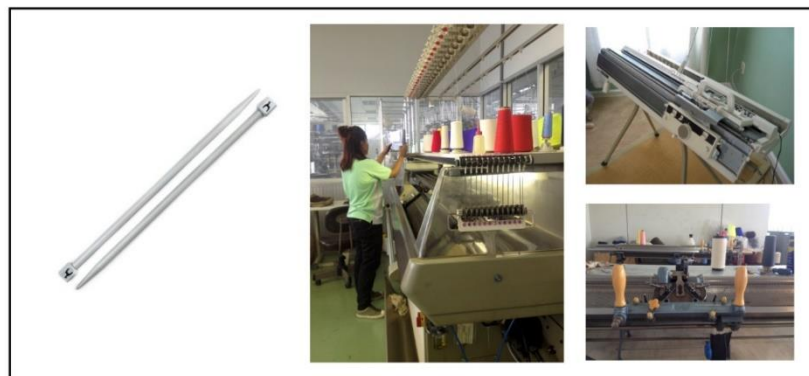
Figure 128 Hand knitting needle (left), automatic knitting machine (center), domestic knitting machine (right top) and V-bed knitting machine (right bellow)
