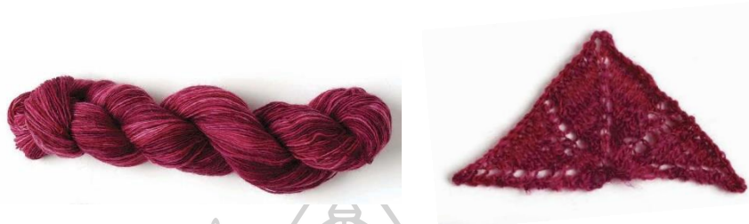
Figure 33 A sample of thin low-twist single yarn (left) and knitted fabric from low-twist single yarn (right) (Amy King, 1973: 71).
