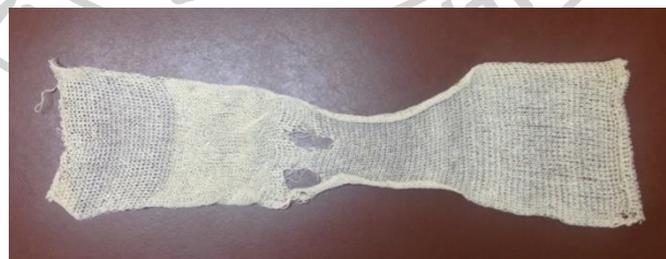
Figure 131 A fabric produce by V-bed knitting machine material : Yarn from cut cocoons sliver, open-end spinning.
