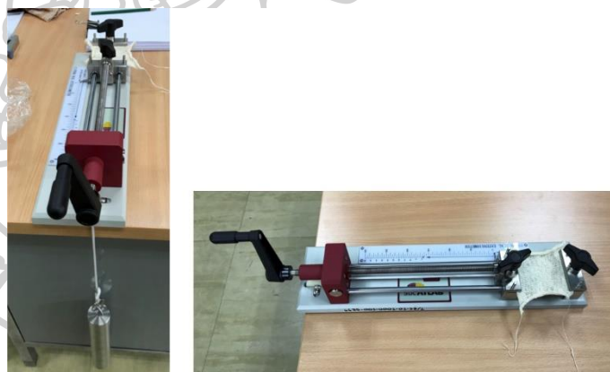
Figure 160 Elasticity testing tool: Fryma Fabric Extensometer
