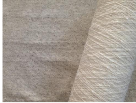
Figure 132 A fabric produce by automatic knitting machine :Shima seike SES.122 multi gauge material : Yarn from 50:50 percentage cut cocoons sliver : cotton sliver.
