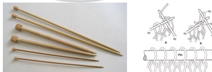
Figure 79 Hand needle (left) and Principle of hand knitting using pin (Sadhan Chandra Ray, 2012:3-4)
