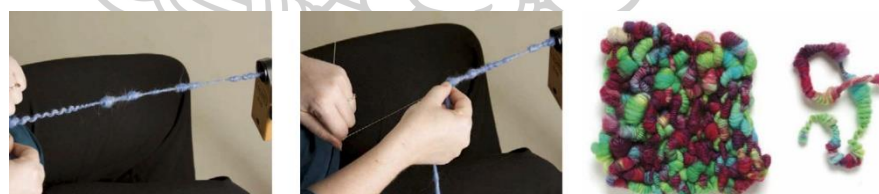
Figure 44 The bobble yarn processing (left) and a sample of knitted fabric (right) (Amy King, 1973: 103).
