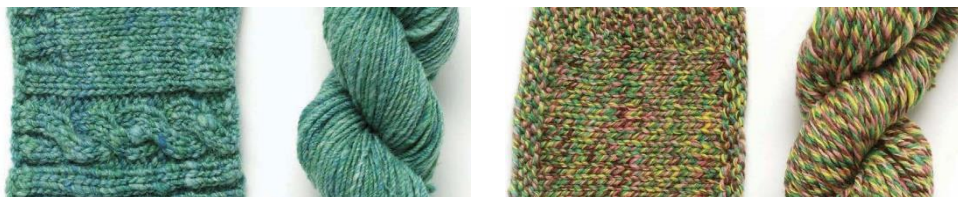
Figure 38 The sample of Woolen Three-ply yarn and knitted fabric and Four-ply yarn and knitted fabric (Amy King, 1973: 91)
