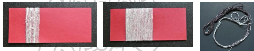
Figure 126 Ring spinning machine: Yarn from cut cocoons sliver (left), open-end spinning machine: Yarn from cut cocoons sliver ( centre) , and open-end spinning machine: yarn from silk fabric waste (purple) (right)
