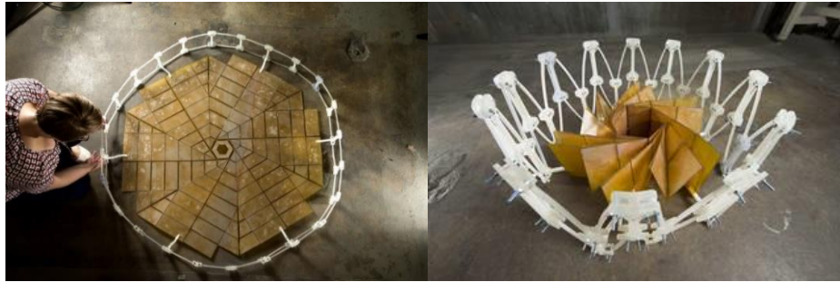
Figure 102 Solar power using the principle of origami
