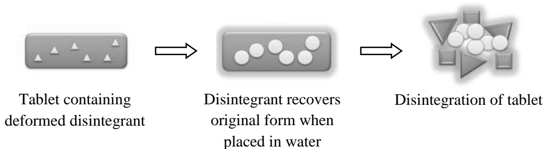
Figure 2.9 Deformation mechanism of a disintegrant.
