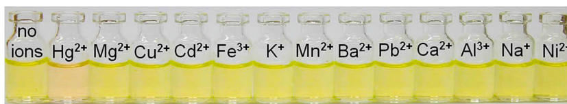
Fig. 9. Chromogenic change of FC4 ( 10.0 \mu\text{M} ) in the absence and presence of \text{Hg}^{2+} , \text{Mg}^{2+} , \text{Cu}^{2+} , \text{Cd}^{2+} , \text{Fe}^{3+} , \text{K}^+ , \text{Mn}^{2+} , \text{Ba}^{2+} , \text{Pb}^{2+} , \text{Ca}^{2+} , \text{Al}^{3+} , \text{Na}^+ and \text{Ni}^{2+} ( 45.0 \mu\text{M} ).
