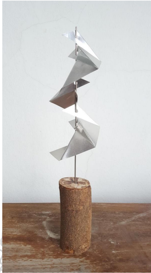
Figure 68. Tilted blade allow one side to pick up the wind better than the other side, so it could rotate easily. By Researcher.
