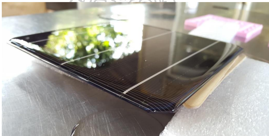
Figure 51. Coating the photovoltaic cell with resin to prevent damage. By Researcher.
