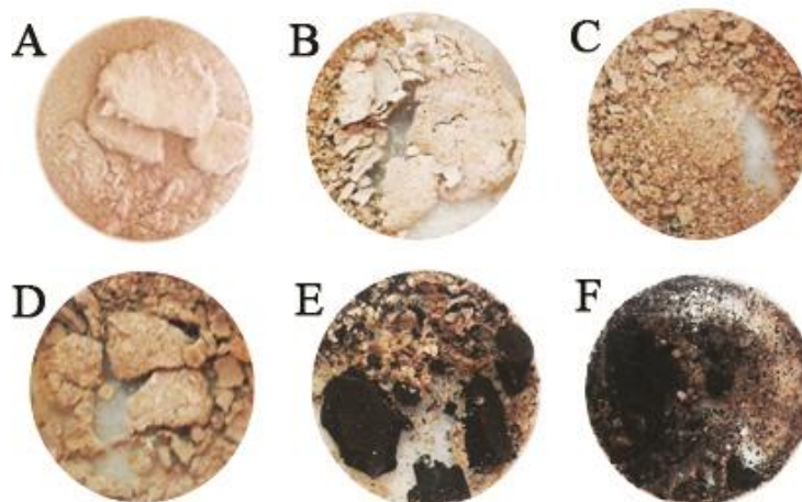
Figure 22 Six fractions including (A) fraction E4W, (B) fraction E4N1, (C) fraction E4N2, (D) fraction E4N3, (E) fraction E4N4, and (F) fraction E4N5 were separated from fraction E4 by using DEAE FF anion chromatography column (5 mL), eluted with step concentration of NaCl (0, 0.05, 0.1, 0.2, and 0.5M).
