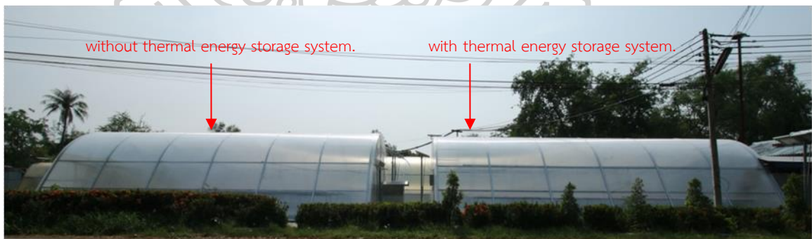
Fig 29 Parabolic greenhouse solar dryer equipped with thermal energy storage system and without thermal energy storage
