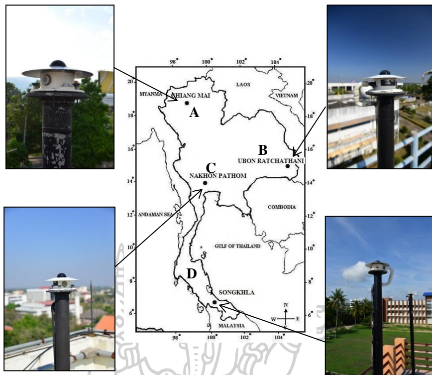
Fig. 11 Position of SNIR measurements and pictorial view of SNIR pyranometers. A, B, C and D indicate the northern, northeastern, central and the southern regions, respectively.
