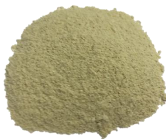
Figure 16 The image of 3%Co/MgO catalyst obtained from wet impregnation method.
