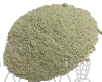
Figure 17 The image of 3%Cu/MgO catalyst obtained from wet impregnation method.
