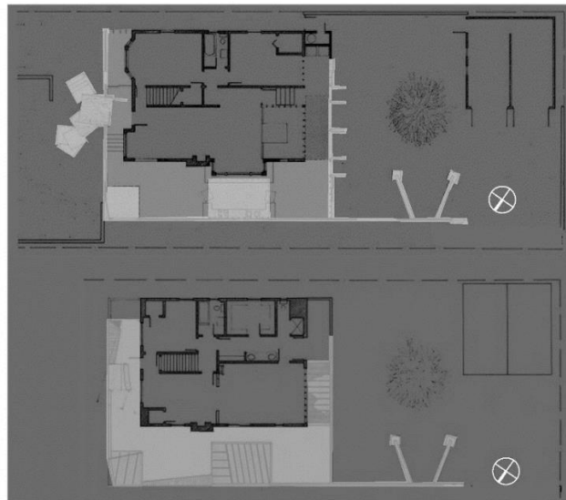
Figure 104: Gehry's 1977-78 Santa Monica Residence; the dualistic difference between the incomplete appearance of original house (darkened) versus the physical extent of the Deconstructivist expansion (lightened); the plan views of the lower and upper levels.
