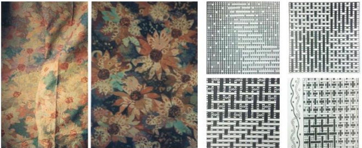
Figure 62: Jacquard woven design and weaves structure pattern Pattern Design by the researcher at Satin Textiles Co., Ltd. (1991)
