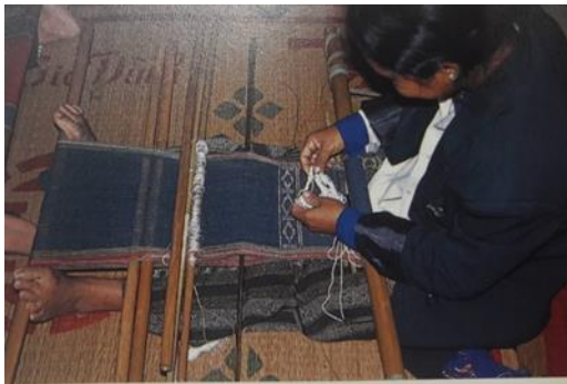
Figure 8: Demonstrating weaving on a foot – braced Backstrap loom.
