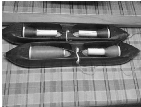
Figure 14: The shuttle a tool for the thread of the weft yarn.
