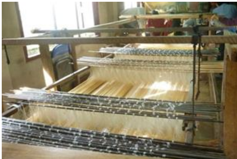
Figure 130: The overview of weaving apparatus of Pha Yok Thong in Surat Thani Province on silk brocade called Pha Mai Phum Riang. It is difference form of drawloom in Surin Province or the weaving apparatus (string model) all Isan area, but it similar Lamphun Province.
