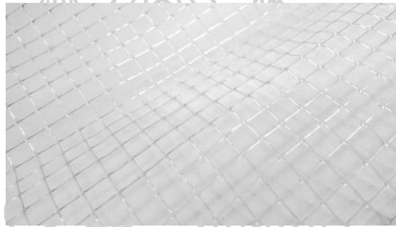
Figure 173: The cotton mesh: The fabrics have moderate densities in both 1/8"square configurations. The strength of the material to be used with artificial fibers. Flexibility to withstand light and water.
