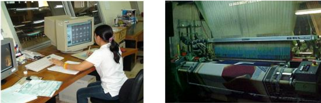
Figure 61: Jacquard Computer Design and Computer Jacquard Rapier Loom
