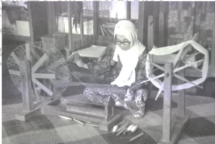
Figure 19: The unwinding a hank of thread and simultaneously winding the threads on to a bobbin. Some threads are used mainly for weft yarn in the filling carrier of fabric.
