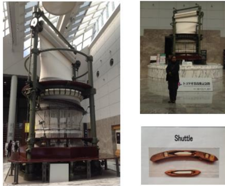
Figure 63: In 1894, Sakichi Toyoda invented the developing a power loom highly efficient Toyoda winding machine. This was an epoch-making development. The Circular looms and a Shuttle curved for weaving the basic plain weave.
