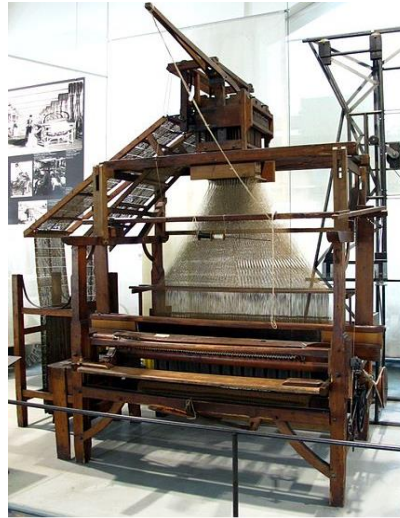
Figure 58: Joseph Marie Jacquard pattern weaving Loom (1804). The older Jacquard drawlooms and punched cards at Deutsches Museum, Munich, Germany.
