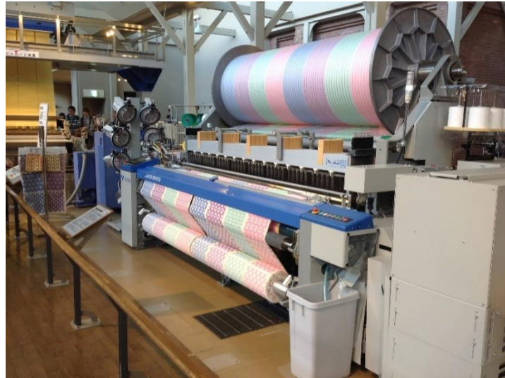
Figure 56: Dobby Weave in program and a woven fabric pattern on loom.
