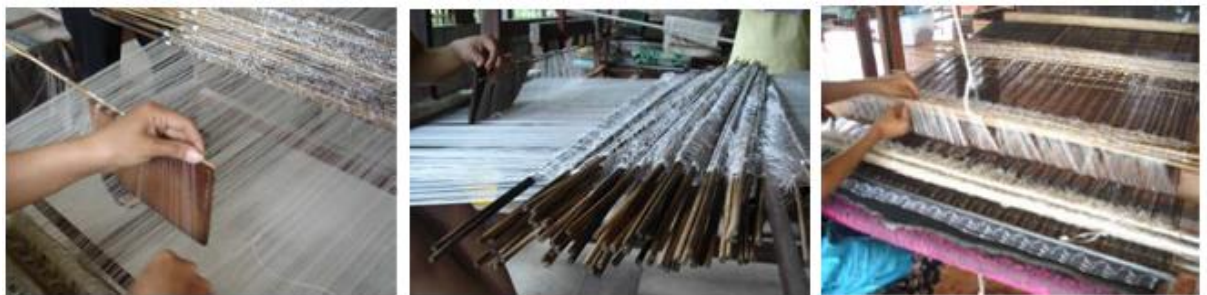
Figure 90: The process of the features and exotic heddle- finishing technique with the supplementary warp of Lamphun Province.
