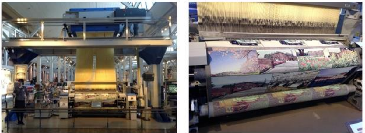
Figure 60: The machine models of Toyota the new air jet Jacquard mechanical looms.
