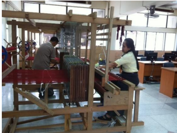
Figure 86: The weaving Dobby loom basic study of Pha Yok Dok in class of computer design.
