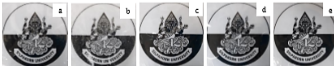
Figure 4. Digital images: a) pure PVA, b) PVA/MFC, c) PVA/1000 rpm, d) PVA/1300 rpm, and e) PVA/1600 rpm
