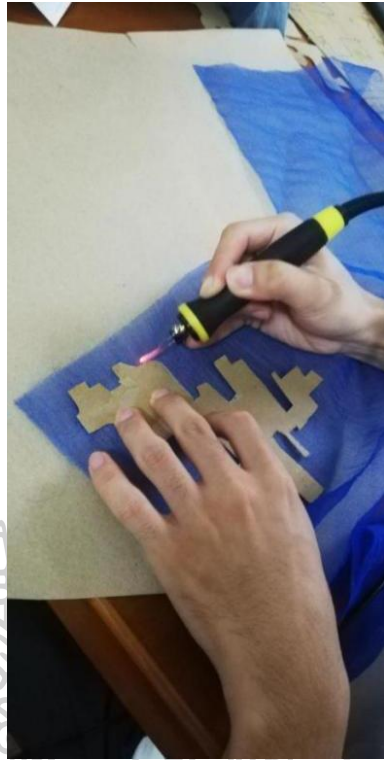
Figure 155 Using a hot melt gun, the lace fabric is reproduced to the same shape as each cardboard.
