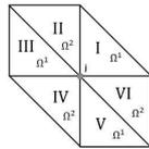
$$A_1 = \int_0^1 \int_0^{1-\eta} 2 \left[ \left( \frac{\partial \tilde{\lambda}_1}{\partial \xi} \right)^2 + \left( \frac{\partial \tilde{\lambda}_1}{\partial \eta} \right)^2 + \left( \frac{\partial \tilde{\lambda}_2}{\partial \xi} \right)^2 + \left( \frac{\partial \tilde{\lambda}_2}{\partial \eta} \right)^2 + \left( \frac{\partial \tilde{\lambda}_3}{\partial \xi} \right)^2 + \left( \frac{\partial \tilde{\lambda}_3}{\partial \eta} \right)^2 \right] d\xi d\eta$$
