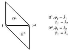
$$A_1 = \int_0^1 \int_0^{1-\eta} 2 \left( \frac{\partial \tilde{\lambda}_2}{\partial \xi} \frac{\partial \tilde{\lambda}_1}{\partial \xi} + \frac{\partial \tilde{\lambda}_2}{\partial \eta} \frac{\partial \tilde{\lambda}_1}{\partial \eta} \right) d\xi d\eta = -1.$$
