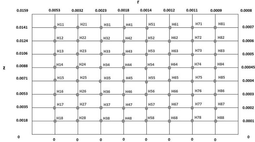
Figure 3.2: Discretizing the domain  $\Omega$  using a uniform grid.
