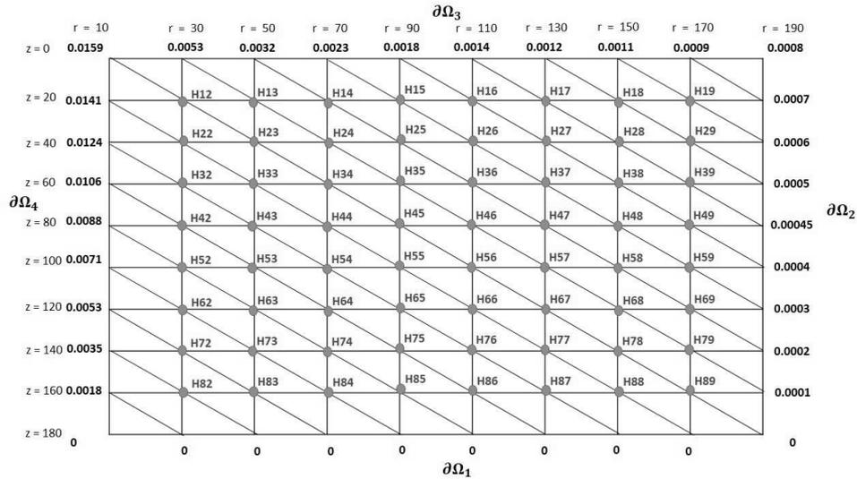
Figure 4.14: Discretizing the domain  $\Omega$  using a triangular uniform grid.
