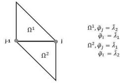
$$A_1 = \int_0^1 \int_0^{1-\eta} 2 \left( \frac{\partial \tilde{\lambda}_1}{\partial \xi} \frac{\partial \tilde{\lambda}_2}{\partial \xi} + \frac{\partial \tilde{\lambda}_1}{\partial \eta} \frac{\partial \tilde{\lambda}_2}{\partial \eta} \right) d\xi d\eta = -1.$$
