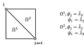
$$A_1 = \int_0^1 \int_0^{1-\eta} 2 \left( \frac{\partial \tilde{\lambda}_2}{\partial \xi} \frac{\partial \tilde{\lambda}_3}{\partial \xi} + \frac{\partial \tilde{\lambda}_2}{\partial \eta} \frac{\partial \tilde{\lambda}_3}{\partial \eta} \right) d\xi d\eta = 0.$$
