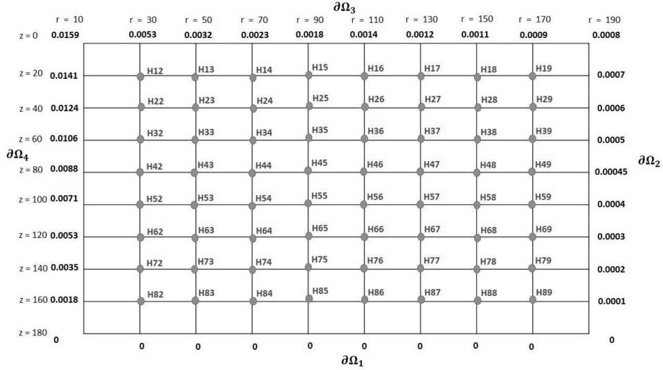
Figure 4.1: Discretizing the domain  $\Omega$  using a rectangular uniform grid.
