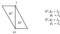
$$A_1 = \int_0^1 \int_0^{1-\eta} 2 \left( \frac{\partial \tilde{\lambda}_1}{\partial \xi} \frac{\partial \tilde{\lambda}_3}{\partial \xi} + \frac{\partial \tilde{\lambda}_1}{\partial \eta} \frac{\partial \tilde{\lambda}_3}{\partial \eta} \right) d\xi d\eta = -1.$$
