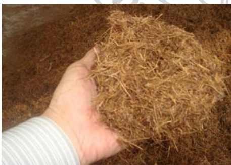
Figure 108 Shredded EFB to pulp (Gemco Energy, 2021).
