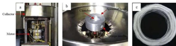
Fig. 1. (a) Rotational jet spinning machine; (b) spinneret head and collector; (c) non-woven micro fiber mat
