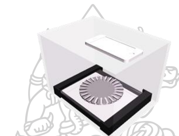
Figure 15. Image capture setting of smartphone-based ion-pair extraction.
