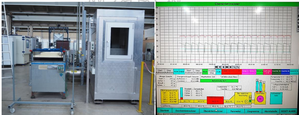
Figure A1 Schematic diagram of the laboratory-made hot air dryer, drying compartment, and controlling program used in the experiments.
