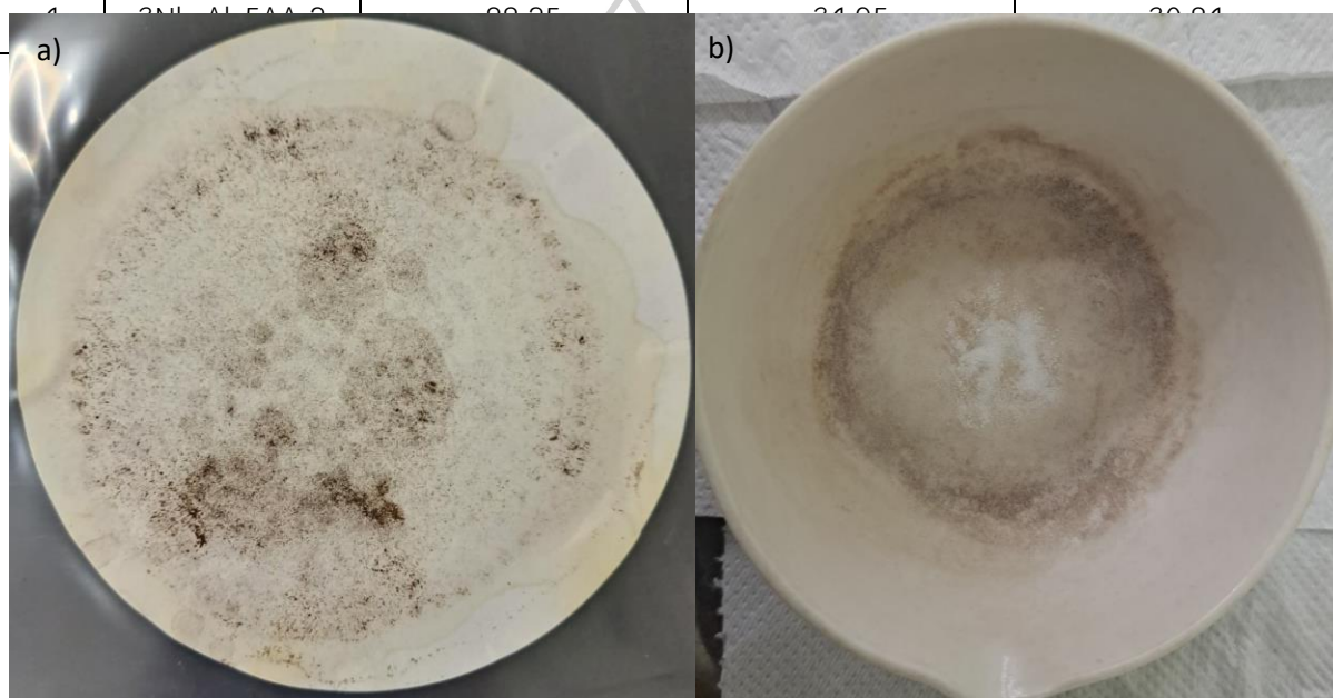
Figure 24 catalysts after the reaction test (a) and catalysts after pretreatment (b)
