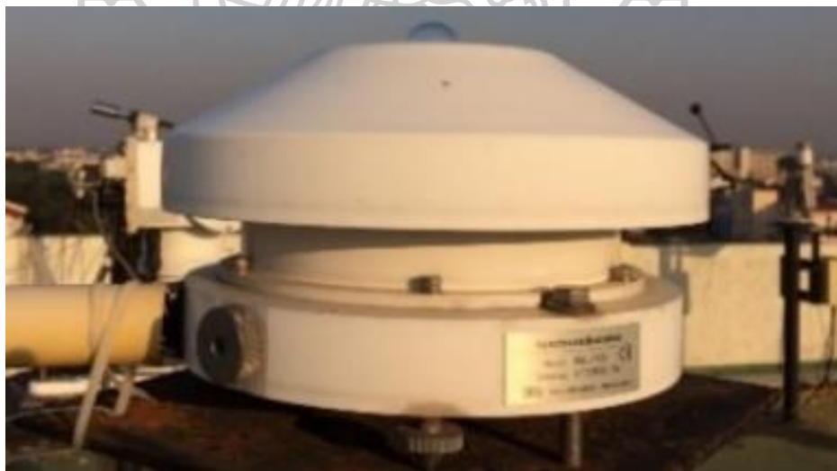
Figure 1. EKO MS-710 spectroradiometer installed at Nakhon Pathom station.
