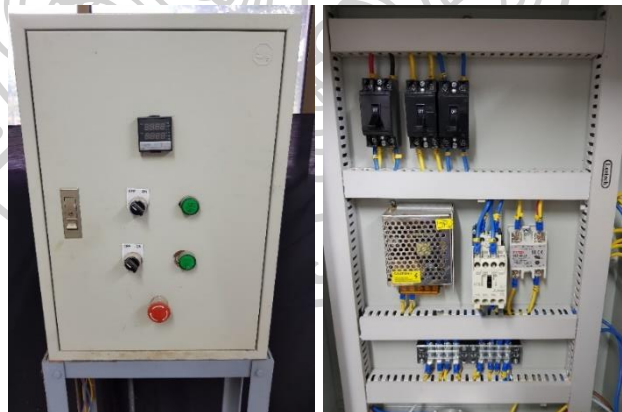
Fig. 23 The electrical control cabinet, outside (left), inside (right).
