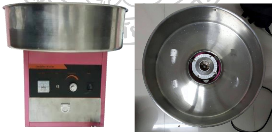
Fig. 10 The cotton candy machine was the basis of the rotational jet spinning machine (RJS).
