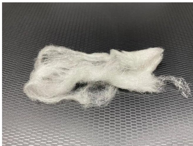
Fig. 44 Polylactic acid 3052D fiber spun with a condition, 3000 rpm, and 240 °C.
