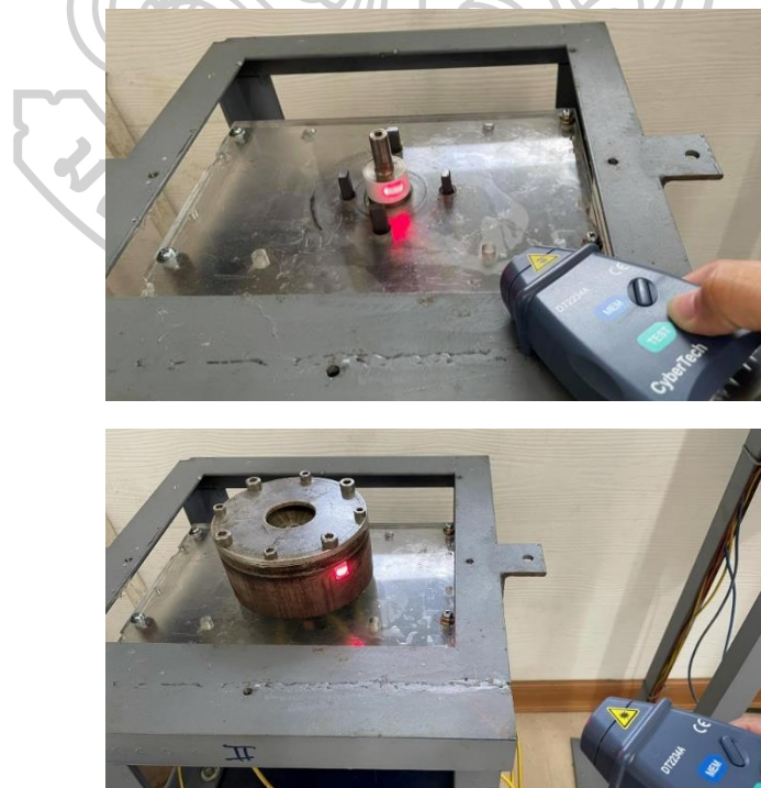
Fig. 36 The position testing, without the spinneret (top), with the spinneret (bottom).
