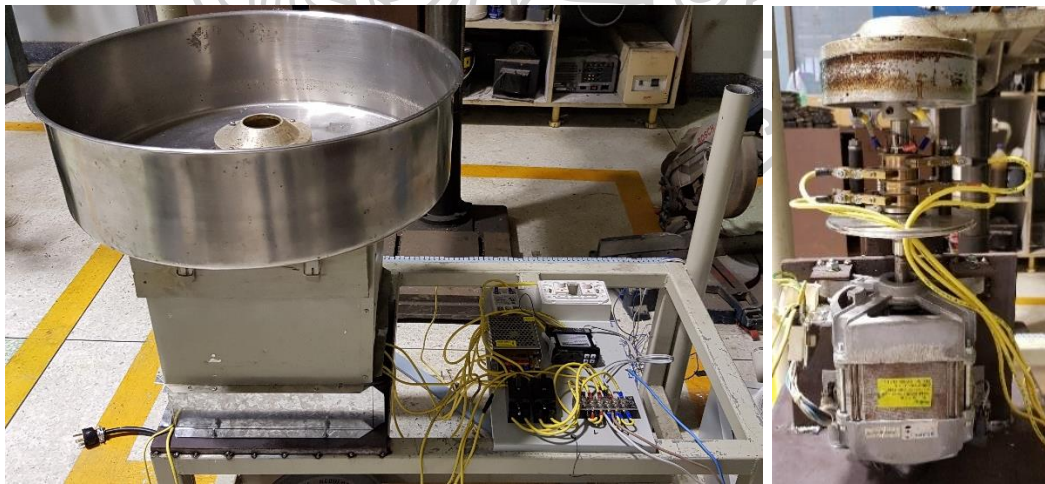
Fig. 17 The rotational jet spinning machine (left), slip ring, and a motor were assembled (right).
