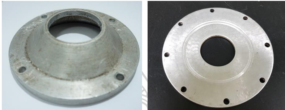
Fig. 20 The cover before reducing the thickness (left) the cover after reducing the thickness (right).
