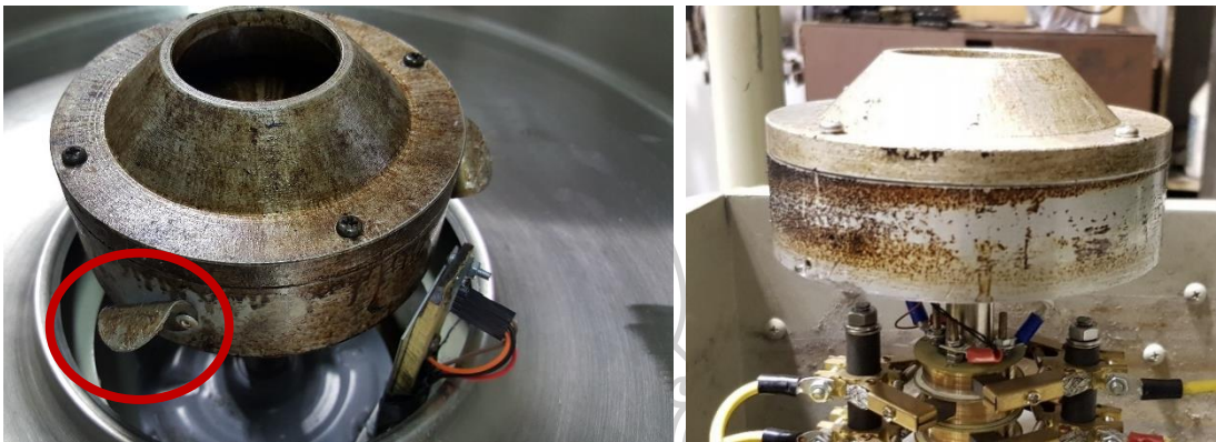
Fig. 16 The propeller installed on the spinneret (red circle, left), the propeller uninstalled on the spinneret (right).
