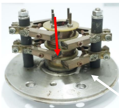
Fig. 15 Slip ring (red arrow) and carbon brush (white arrow).
