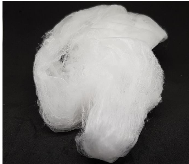
Fig. 18 Polymeric acid non-woven fiber with a condition of 1800 rpm and 190 °C.
