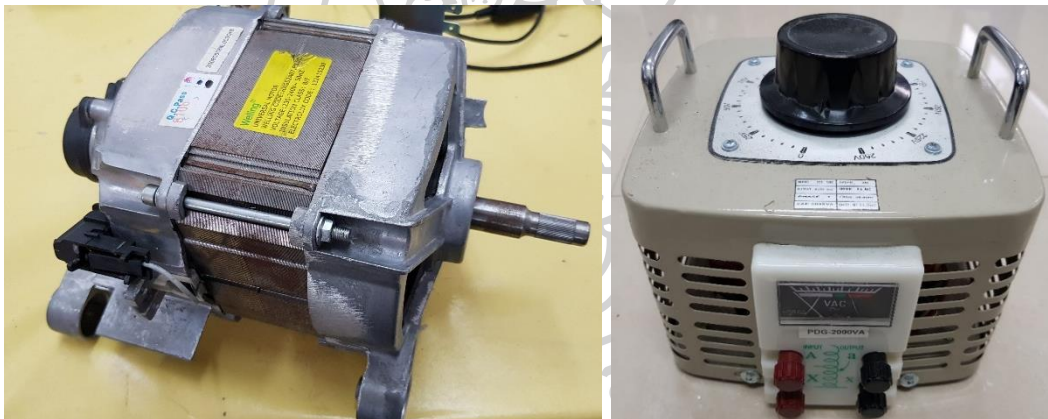
Fig. 13 Universal motor (left) and voltage regulator (right).
