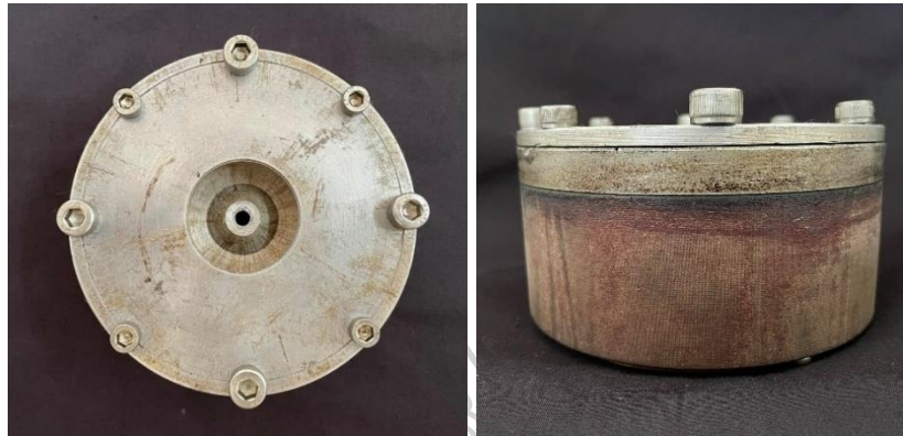
Fig. 32 The spinneret and a cover, top view (left), side view (right).
