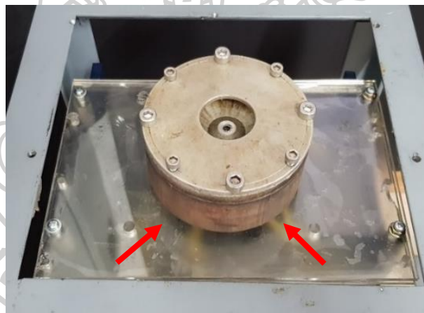
Fig. 33 Spinneret connected to universal motor and carbon brush underneath the spinneret (red arrow).
