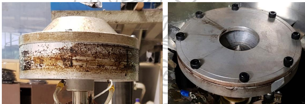
Fig. 21 The spinneret before reduced the unnecessary part (left) and the spinneret after reduced the unnecessary part (right).
