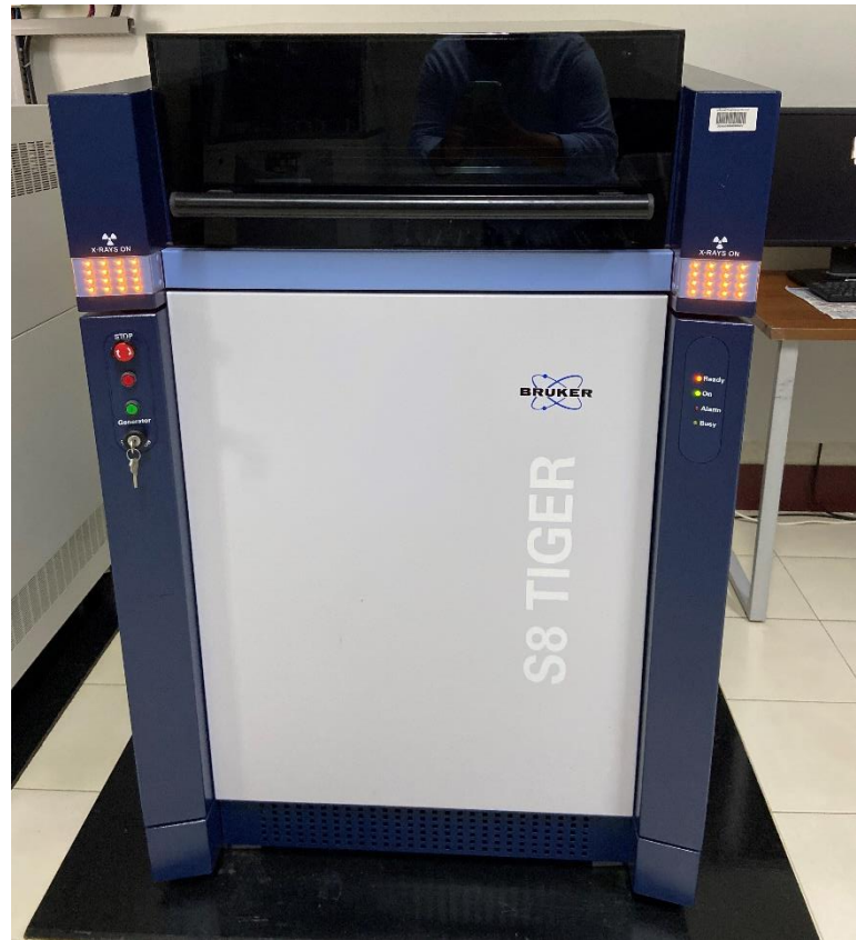
Figure 10 XRF (X-ray fluorescence) model S8 TIGER, Bruker
