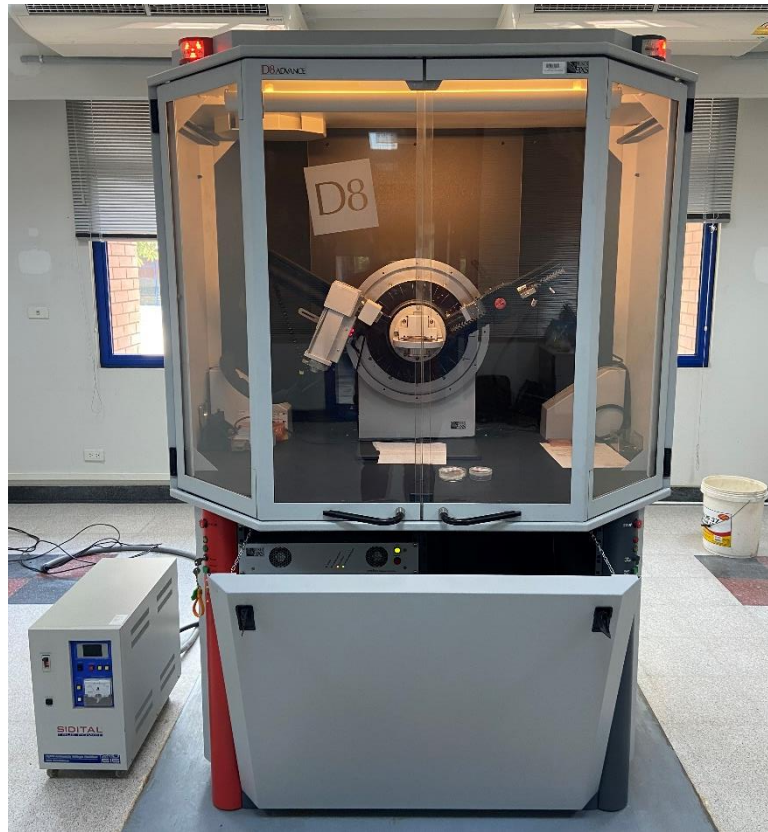
Figure 6 XRD (X-ray diffraction) model D8 Advance, Bruker
