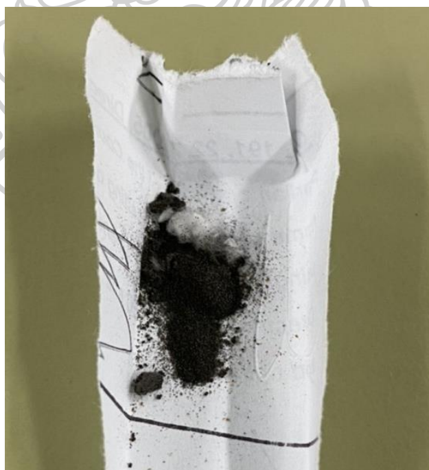
Figure 36 The appearance of the catalyst after CO 2 -TPD measurement
