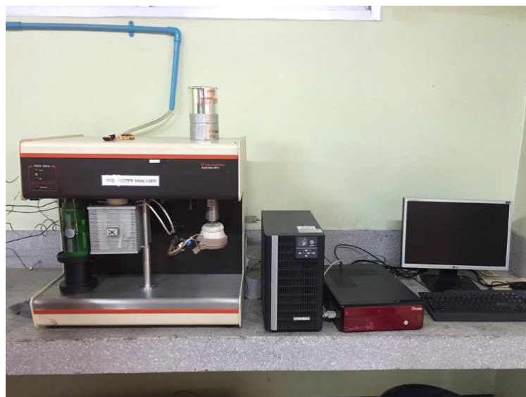
Figure 8 TPD (Temperature Programmed Desorption) instrument (Autpchem 2910 model, Micromeritics)
