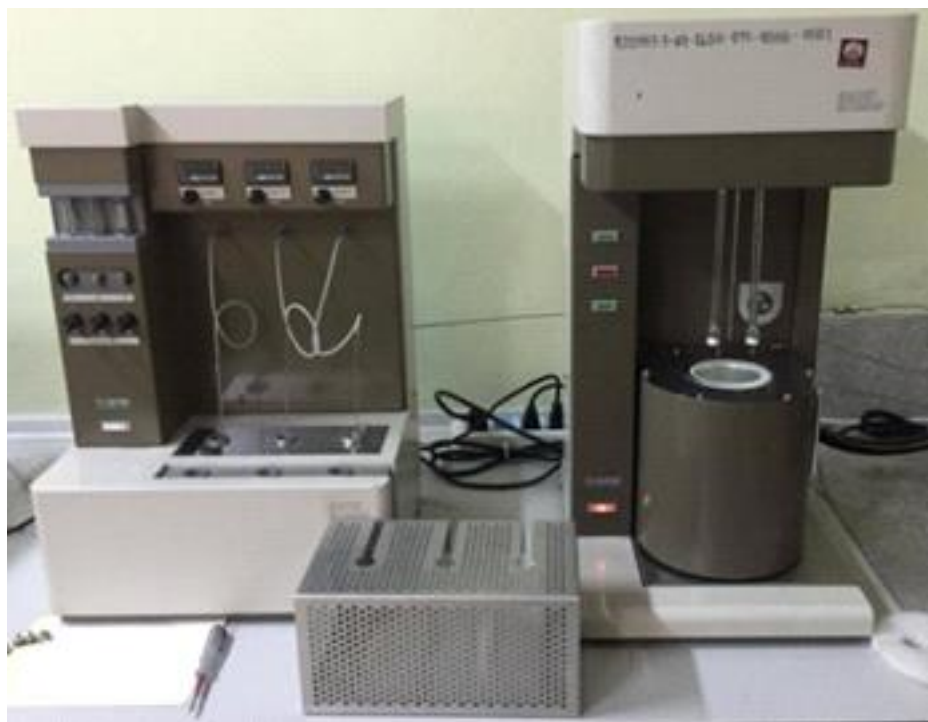
Figure 5 BET (Brunauer-Emmett-Teller) instrument (BELSORP-mini II Microtrac model, BEL Company)
