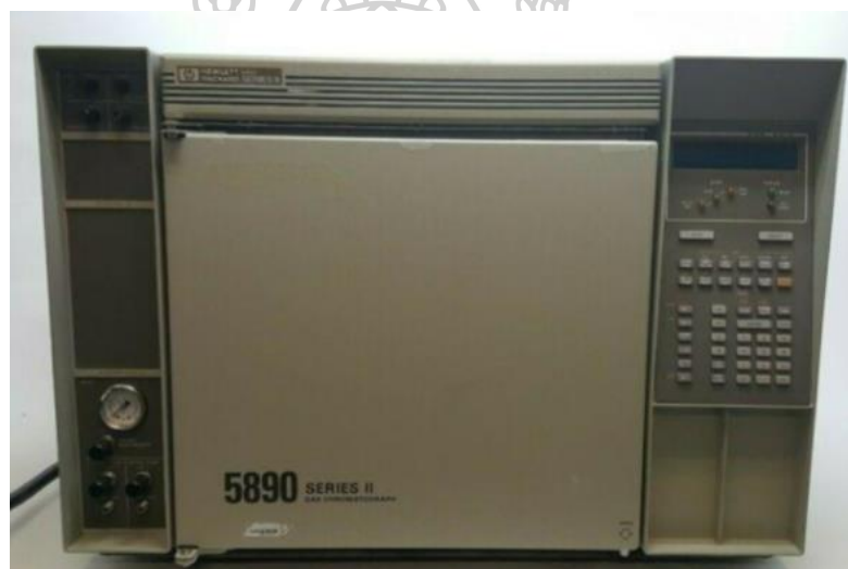
Figure 9 GC-FID (Gas Chromatography-Flame ionization) instrument (HP 5890 series II model)
