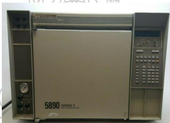
Figure 4.4 GC-FID (Gas Chromatography-Flame ionization) instrument (HP 5890 series II model)
