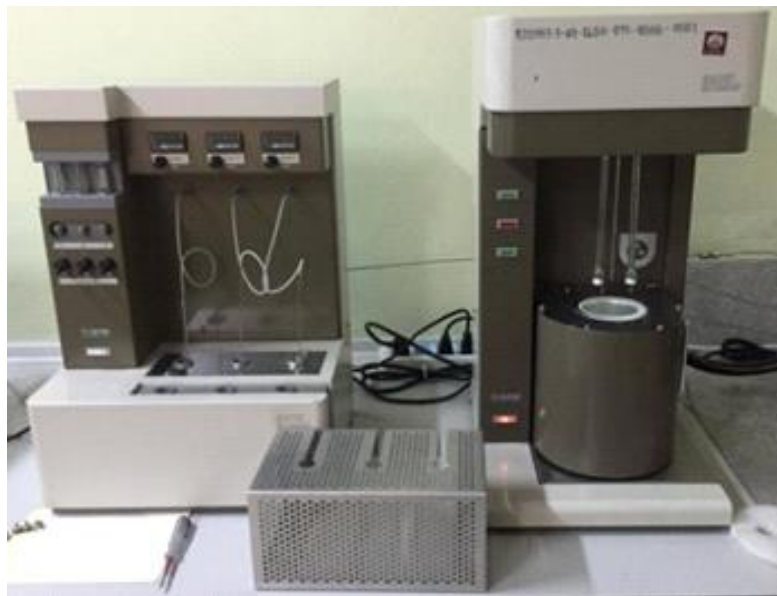
Figure 4.1 BET (Brunauer-Emmett-Teller) instrument (BELSORP-mini II Microtrac model, BEL Company)
