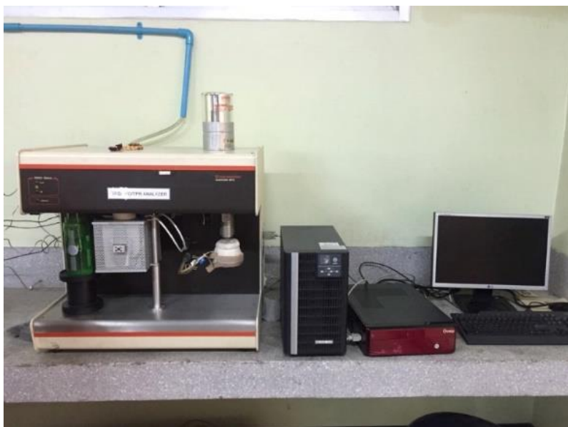
Figure 4.3 TPD (Temperature Programmed Desorption) instrument (Autpchem 2910 model, Micromeritics)
