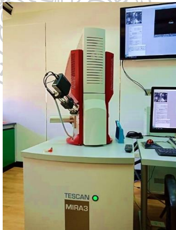
Figure 4.2 SEM (Scanning electron diffraction) instrument (MIRA3 model, TESCAN Company)
