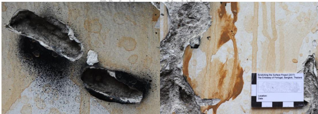
Figure 52 Traces of the aerosol dispersion of the black spray paint Source: Elias Campidell (June 12, 2023)
