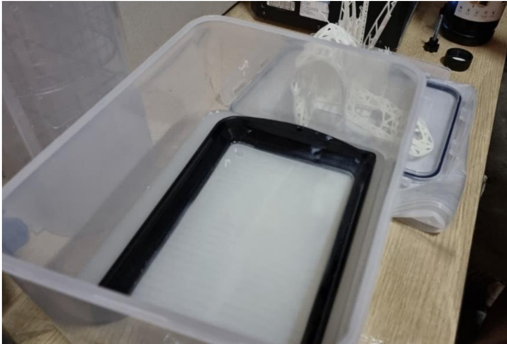
Figure 118 The experimental procedure for 3D printing a parametric chair model is depicted, with the resin cleaning solution
