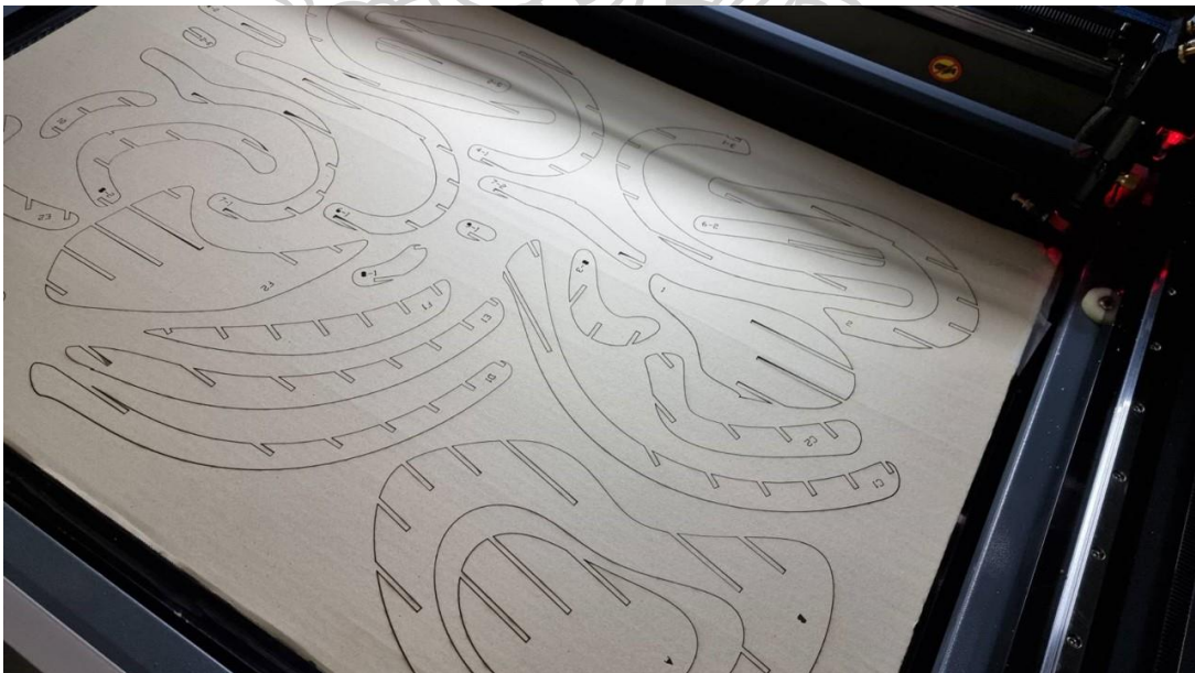
Figure 85 Cardboard material is cut by a laser cutter for further assembly.
