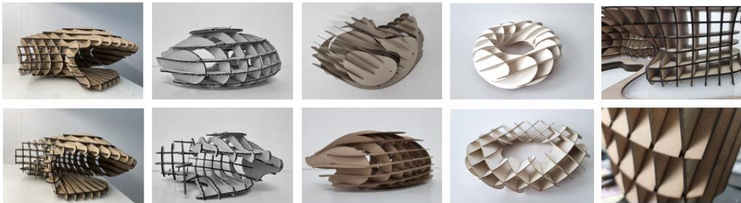
Figure 93 Experimenting with waffle structures with different shapes and materials such as plywood, cardboard, and craft board.
