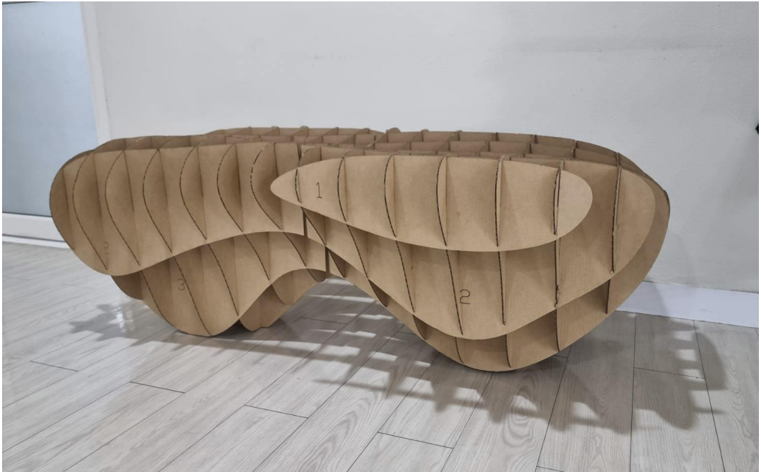
Figure 94 The bench chair model is replicated in real size with a parametric waffle structure design.
