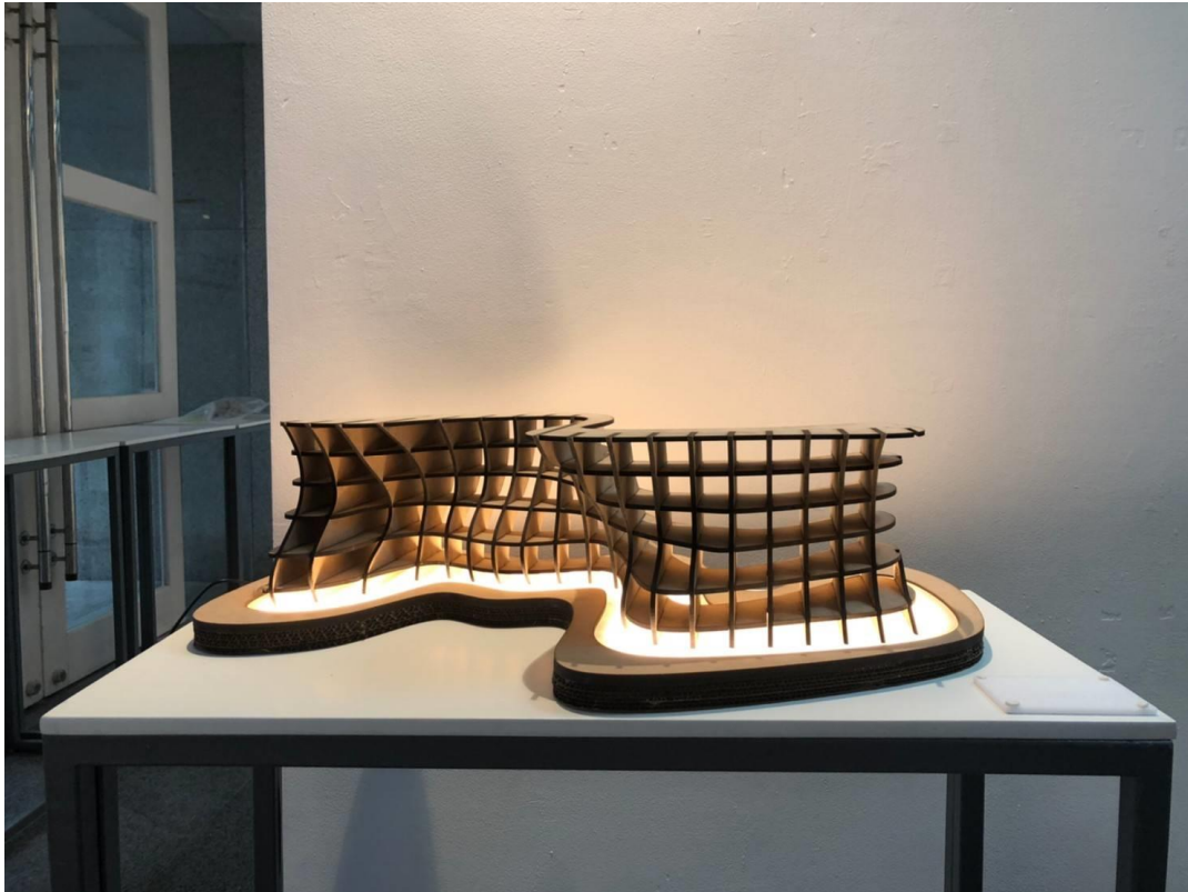
Figure 92 Simulation model for walls with parametric waffle structure design.
