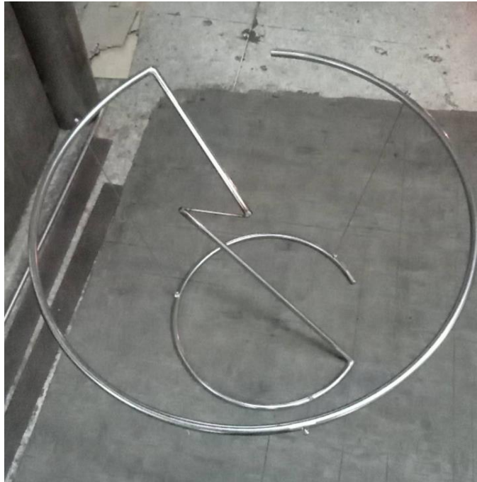
Figure 117 Making a side table frame using wrought iron
