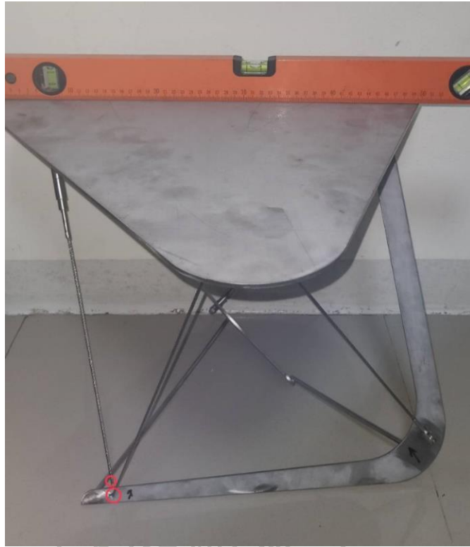
Figure 168 Precisely gauge the water level to ensure that the top of the furniture is positioned accurately at a level of 0 degrees.
