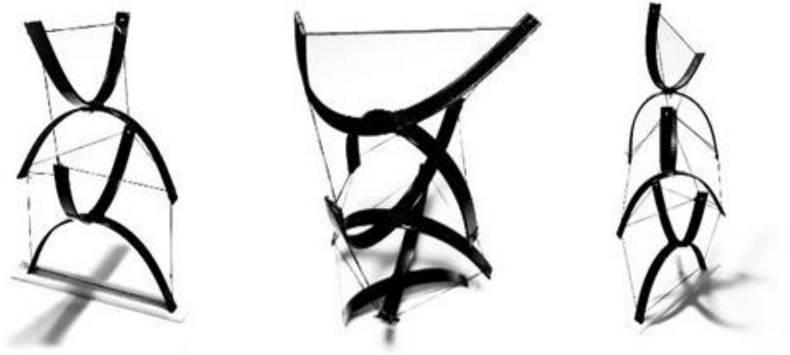
Figure 41 Connection of Linear System Tensegrity Subunit
