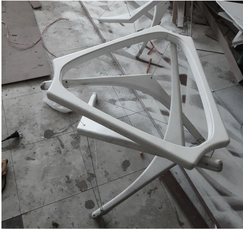
Figure 126 Complete assembly and proceed to the polishing and painting process.
