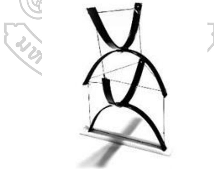
Figure 34 Connection of linear system Tensegrity subunit
