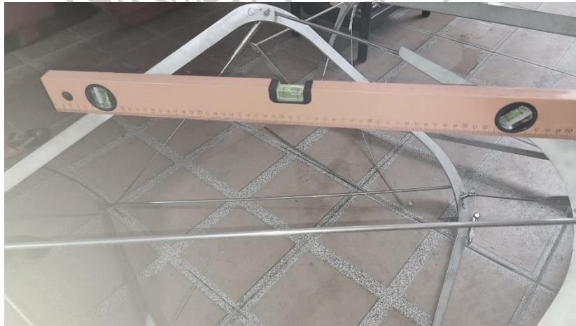
Figure 169 Precisely gauge the water level to ensure that the top of the furniture is positioned accurately at a level of 0 degrees.
