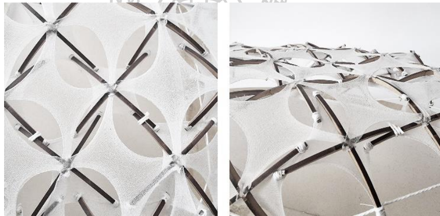
Figure 86 Final Mixed Tensegrity Structure Model
