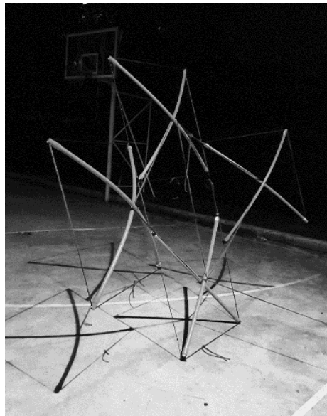
Figure 83 Experimenting with a Full-Scale Physical Model of Tensegrity Structure
