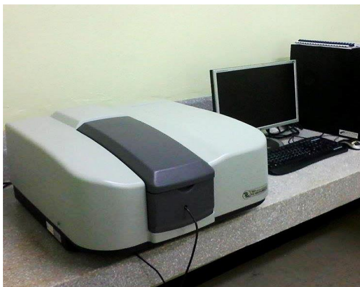
Figure 8 Ultraviolet-Visible (UV-VIS) spectrometer (T92+ UV spectrometer, PG Instruments Ltd., UK)
