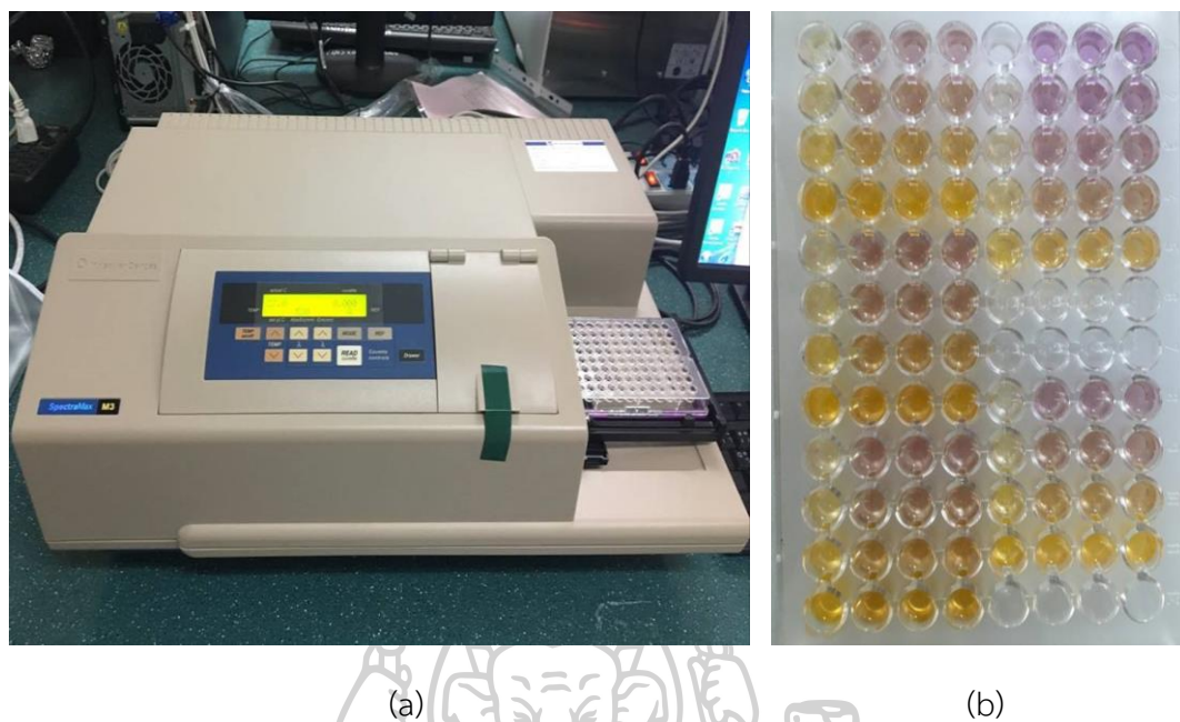
Figure 10 The instrument for analyzing of DPPH free radical scavenging capacity assay; (a) Microplate reader (Spectramax® M3, Molecular devices, USA) (b) 96-wells microplate
