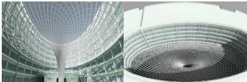
Figure 67 Alternate leaf order morphology was calculated to generate the construction form map Note. Researchers draw their own, 2023
