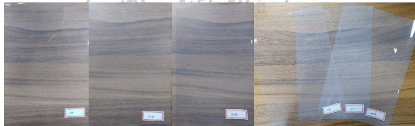
Figure 148 ETFE membrane material
