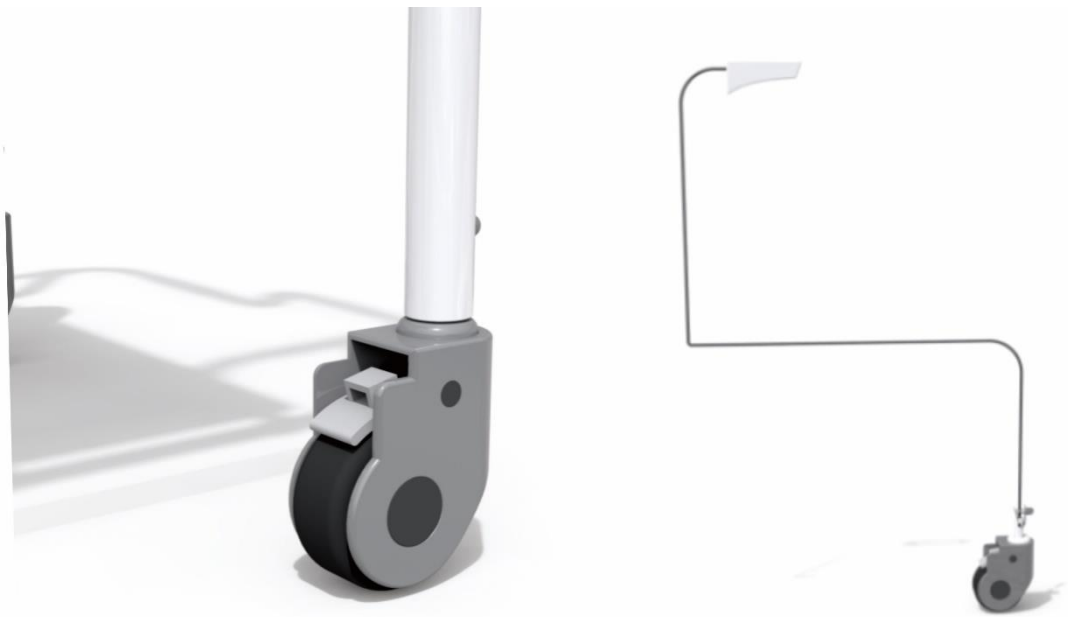
Figure 62 Solution for rotatable wheels and braking system
