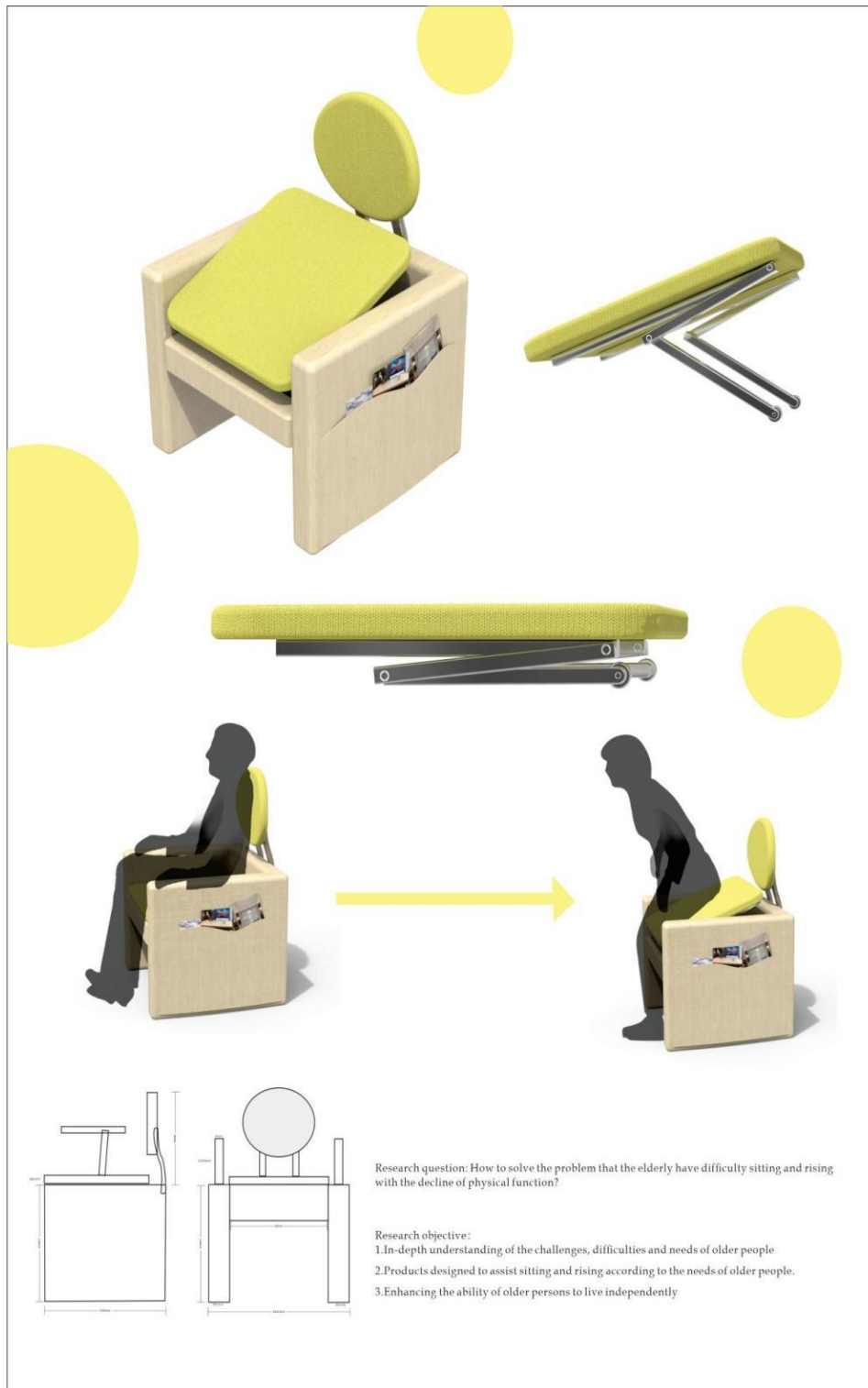
Figure 48 Non-Electric Hydraulic Assist Chair
