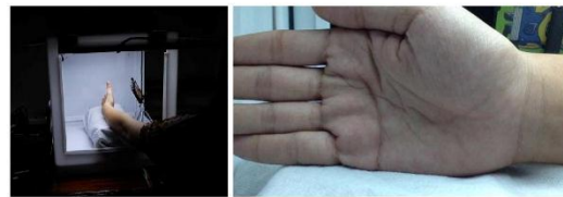
Figure 1 Settings for video acquisition. Left: light-control box and a tripod for holding a tablet. Right: a sample video frame focusing on a palm of a subject.
