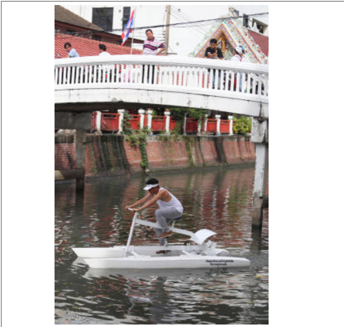
Figure 107 The use of water treatment bike at Khlong Bang Lamphu. The bike idea was obtained from King Bhumibol Chirapattana Low Speed Surface Aerator Model which aims to give oxygen to the water, attract tourists, and enhance the health of the community
